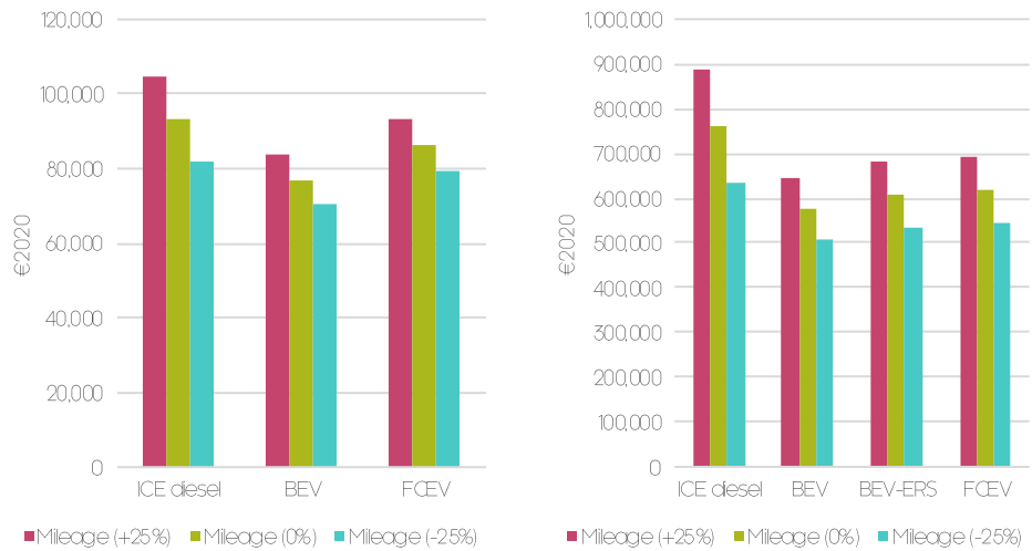
Figure 7.4: Total cost of ownership cost of use sensitivities for vans (left) and HHGVs (right) in 2030
