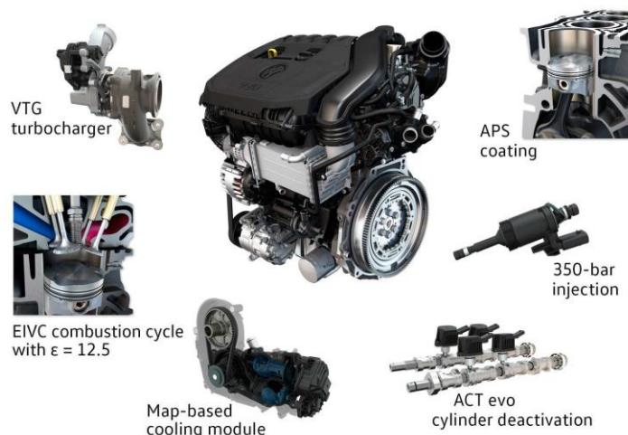
Figure 12 - Examples of technologies fitted on Volkswagen’s new 1.5-litre petrol engine
