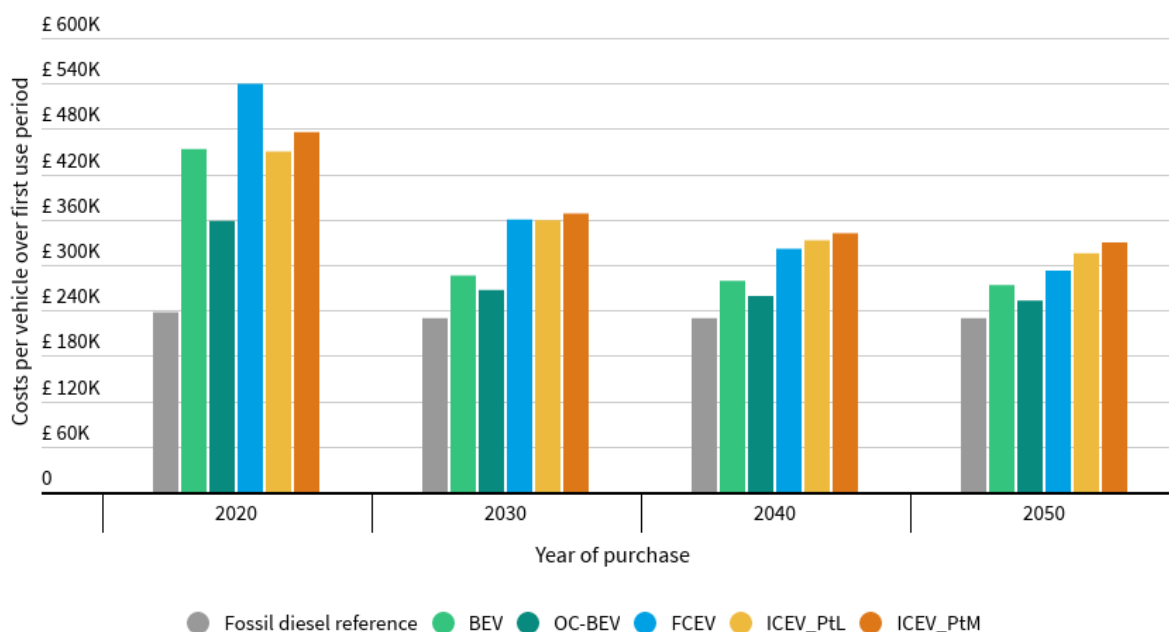
Figure 17: Lifetime system costs - sensitivity analysis with electricity-based fuel production in North Africa
