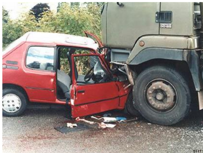
Figure 16: Example of gross underrun.
