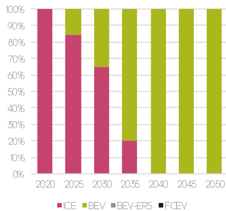
Figure 2.4: Sales mix of HGVs in the TECH BEV scenario (% of annual new vehicle sales)
