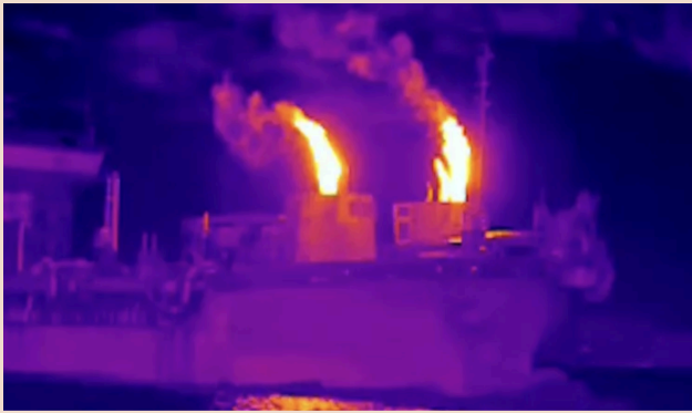
Methane gas slipping from the ship shown on infrared camera
