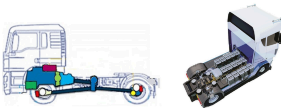
Figure 3. Position of the powertrain in a 4x2 tractor unit with an internal combustion engine (on the left) vs. with an electric motor and battery packs (on the right)
