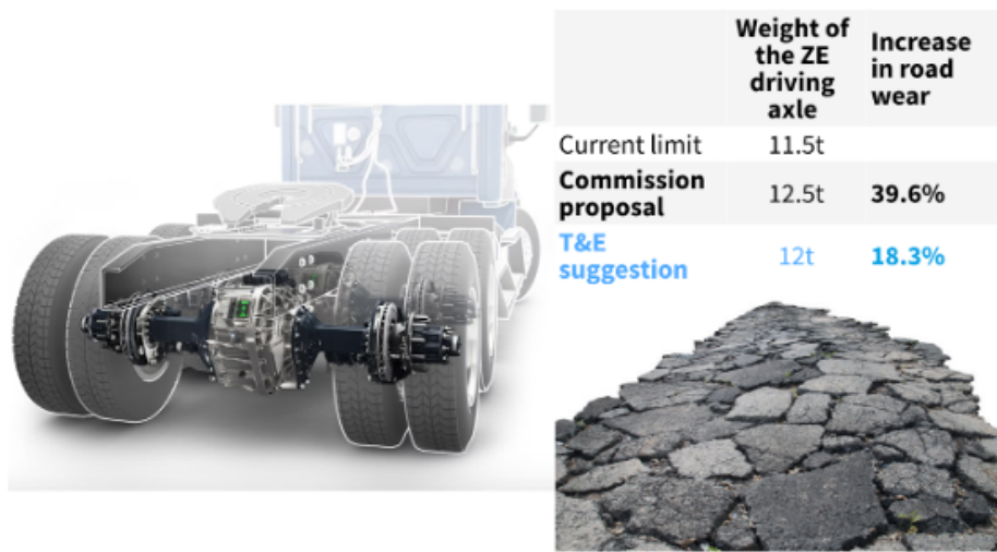
Figure 4. Relation between the increase in the weight of the driving axle and the increase in road wear
