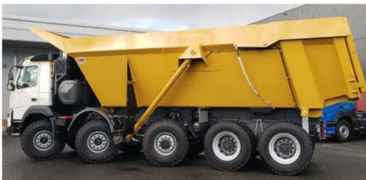
Figure 9. A rigid truck with five axles
