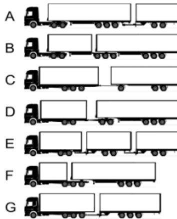
Figure 7. Configurations of European Modular Systems
