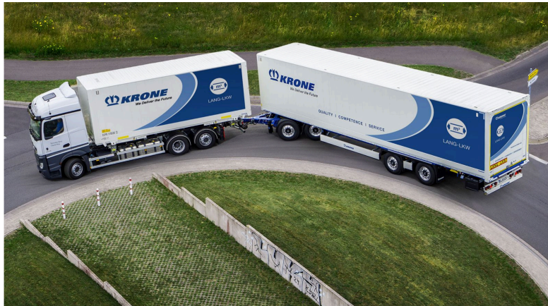
Figure 8. A European Modular System turning a roundabout
