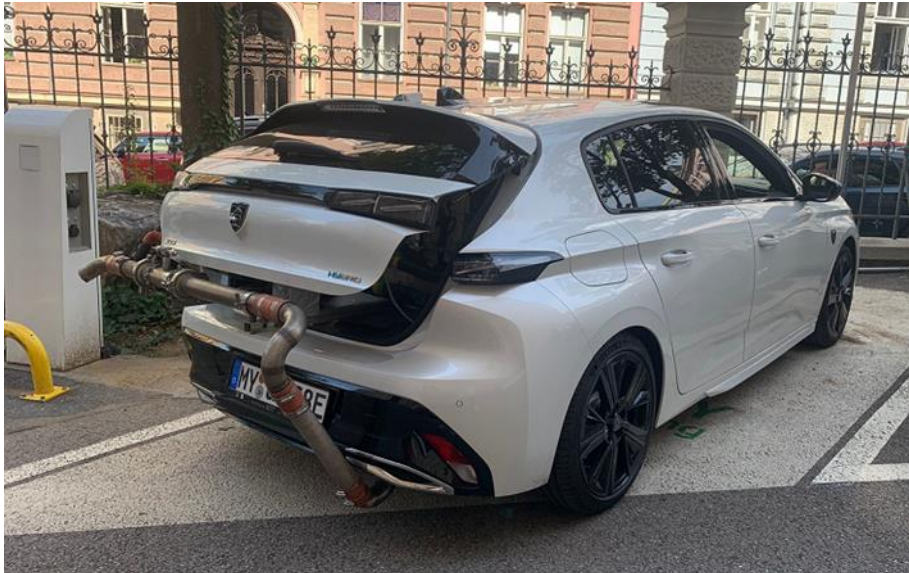
Figure 2.1: Installed PEMS in the Peugeot 308
