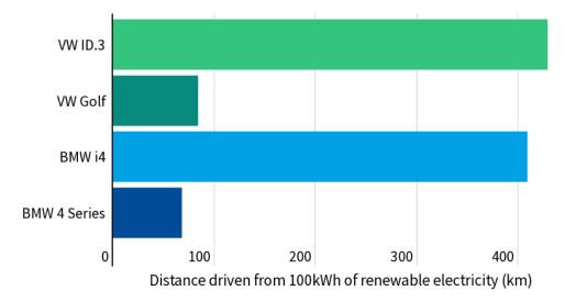
VW Golf and BMW 4-Series ICE driven with pure e-fuel produced from 100% renewable energy **Source**: T&E analysis based on vehicle fuel and electricity consumptions from spritmonitor.de. For ICEs, a 55% e-fuel production efficiency is applied. For BEVs, additional losses include 7% T&D electricity losses, 5% losses from charger equipment and 5% losses from the battery charging efficiency.
