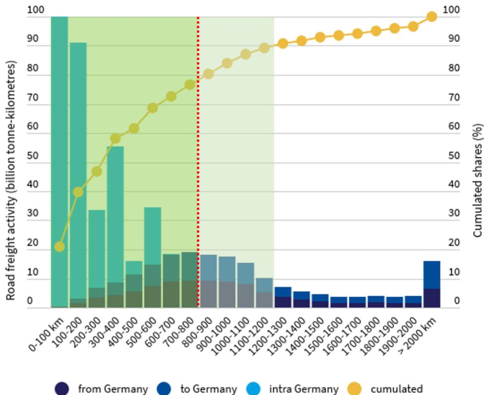
**Notes:** Distribution of road freight activity across vehicle trip distance bands in Germany. Trips can last multiple days. The dark green shade illustrates the activity which can be covered by vehicles with 800 km range without recharging or refuelling. The light green shade extends this coverage based on one recharging or refuelling event during the mandatory daily rest period.
