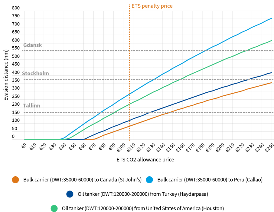
Figure 13: Evasion distance as a function of the semi-full scope ETS price for voyages from/to different ports outside the EU. The y-axis represents the theoretical departure port, with the dotted lines displaying the nautical miles of relevant ports from Ust-Luga
