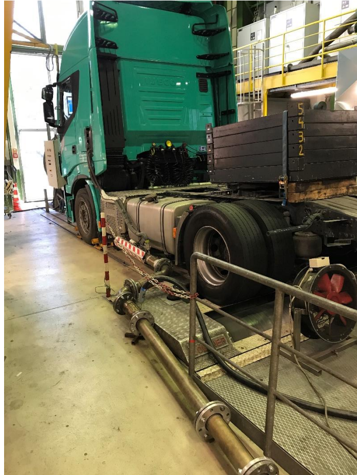
Figure 1: Test vehicle°1, chassis dyno setup
