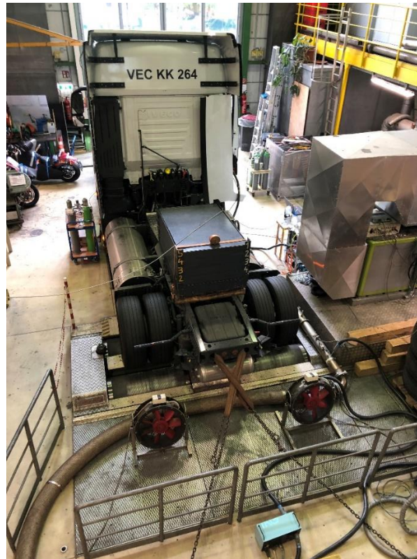
Figure 2: Test vehicle°2, chassis dyno setup
