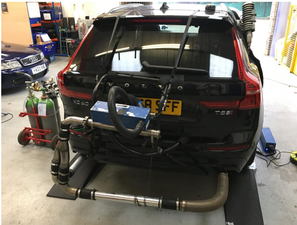
Volvo XC60 undergoing pre-test calibration
