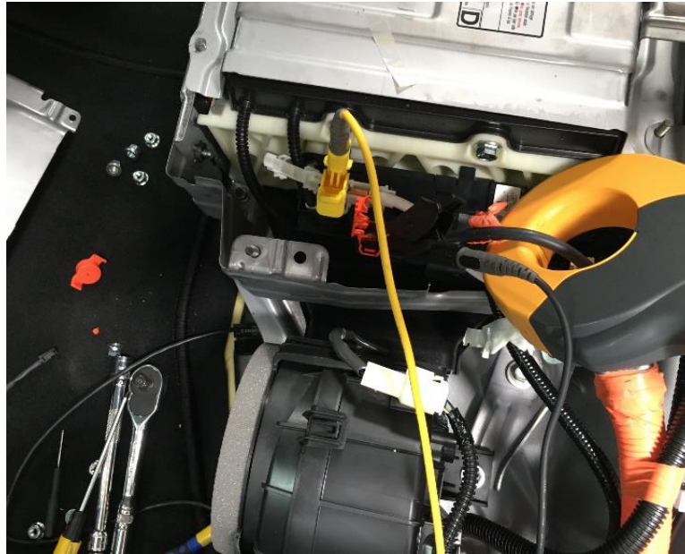
Figure 1 - Battery clamp installed on a test vehicle
