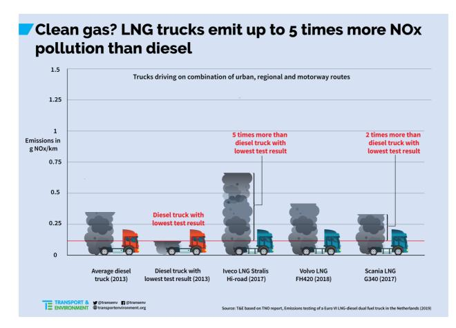
These findings are in strong contrast with the claims made by gas truckmakers (30-35 % less NOx).<sup>xxxv xxxvi</sup> One also needs to take into account that in this testing programme, the latest LNG trucks were compared with older diesel trucks with first generation Euro VI Step A engines from 2013.<sup>xxxvii</sup>
