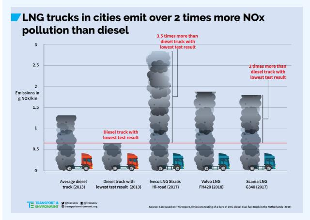
In combined driving (urban, regional and highway) the LNG trucks emit 2 to 5 times more NOx than the diesel truck with the lowest result. If biomethane is used (instead of fossil gas), it does not reduce NOx emissions because the fuel characteristics of biomethane and fossil gas are approximately the same.<sup>i</sup>
