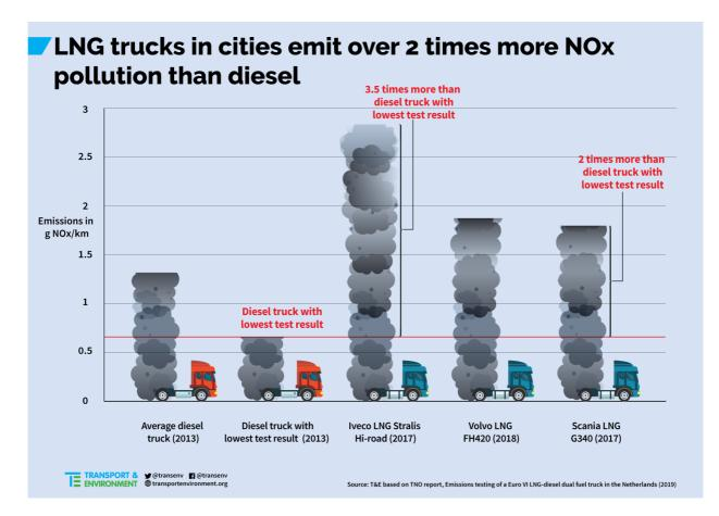
For the Iveco and Scania trucks, only a small share of the higher NOx emissions of LNG trucks is due to the cold start of the engine. Therefore, also during appropriate operating temperatures and acceleration (which happens a lot during stop and go in cities), TNO measured higher NOx emissions for both trucks tested.<sup>xxxiii</sup>
