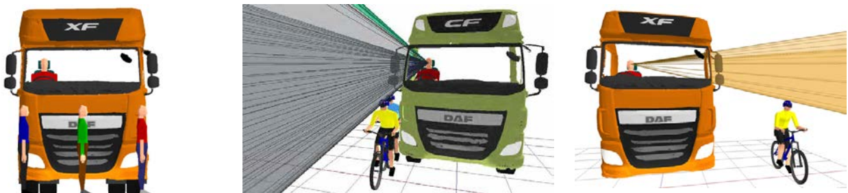
Figure 8: accident configurations analysed by LDS (pedestrian in front of cab, cyclist left & right of cab)
