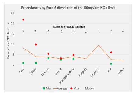
The ICCT research shows Euro 6 emission limits can be met in real-world driving (technology exists and one vehicle complied) but whether they are or not depends on the choice of emission abatement technology and how it is configured within the vehicle. For example the Selective Catalytic Reduction (SCR) technology has been proven to effectively reduce NOx to Euro 6 limits.
