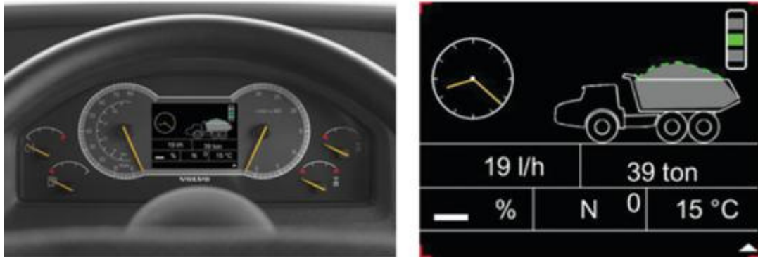
Figure 5: In-vehicle display of the Volvo OBW system
