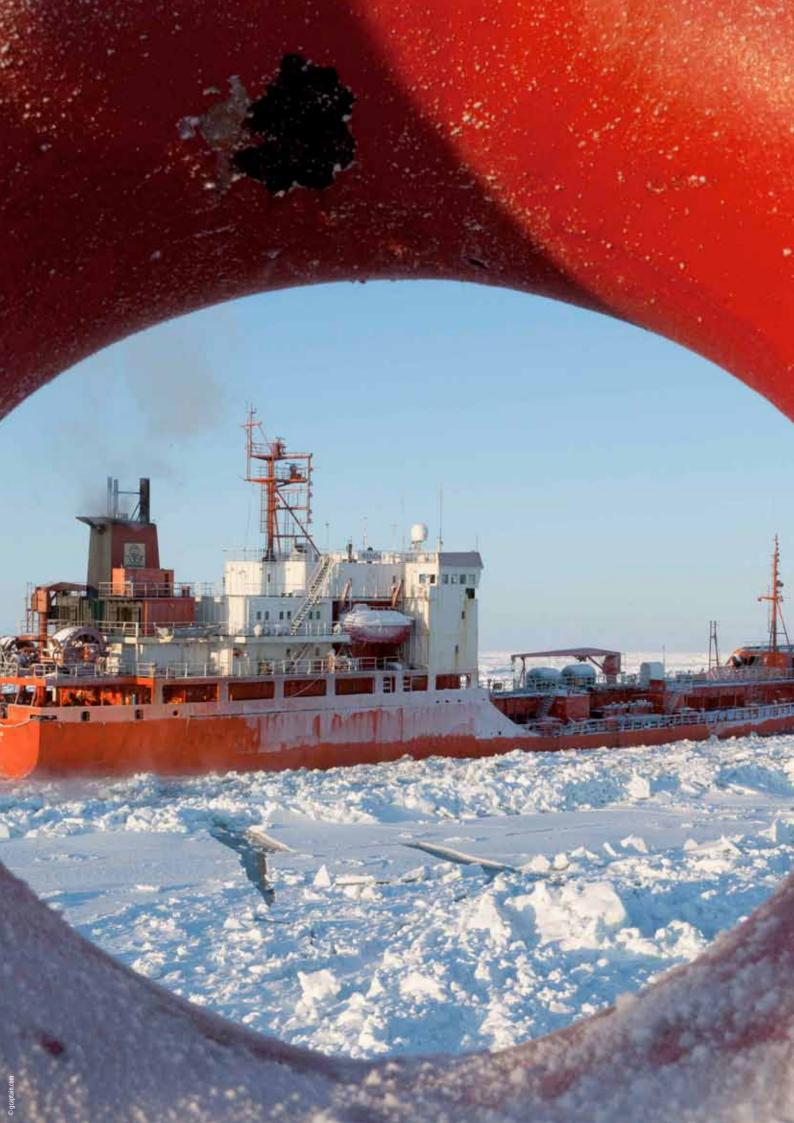
"It is widely acknowledged that the risk of damage to the hull of a ship that is operating in ice is principally a factor of the ice thickness and the speed of the ship in the ice; and that, in general, possible ship structural damage from ship-ice interaction accidents can be avoided if an appropriately safe speed is considered and the ship structure is accordingly strengthened."
