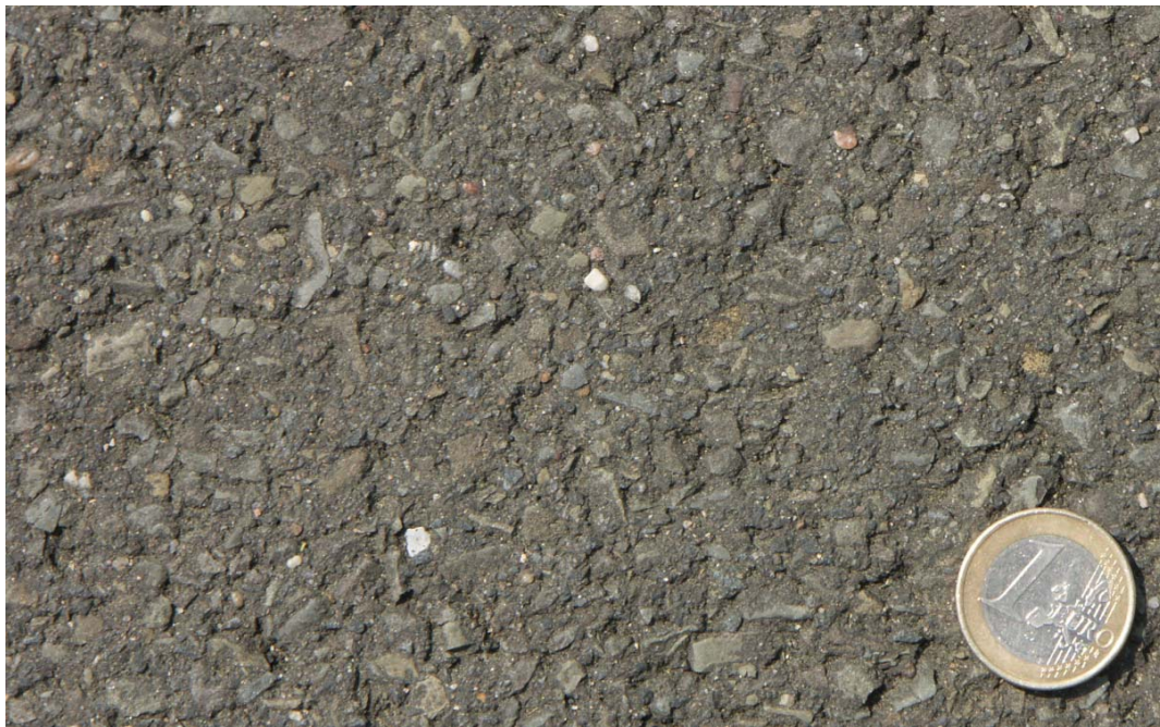
Fig. 27. Illustration of how the texture of a typical reference surface as specified in the Directive and in ISO 10844 may look like. The picture is from the ISO surface at BAST in Bergisch-Gladbach in Germany. The coin is a one Euro coin.
