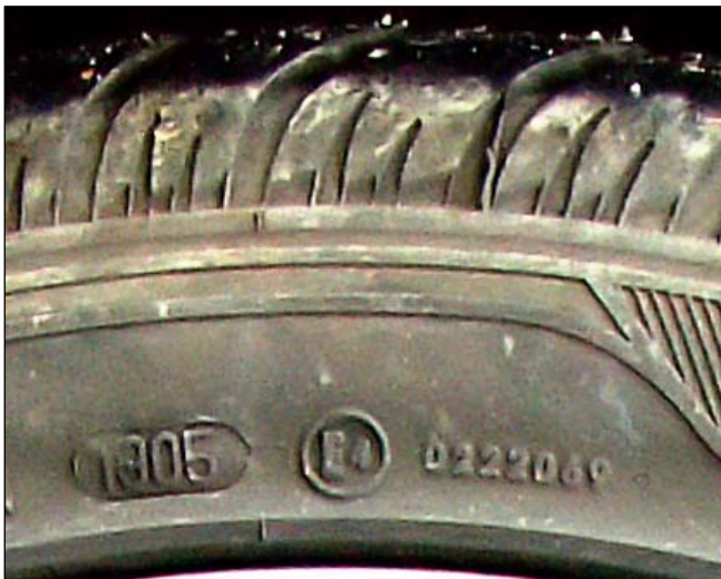
Fig. 7. Example of tyre label moulded into the sidewall.
